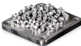
Partial, copings and bridges production in LaserForm CoCr (C)
